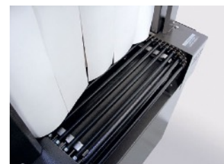
Hi Density Rollers - Tight Spacing
