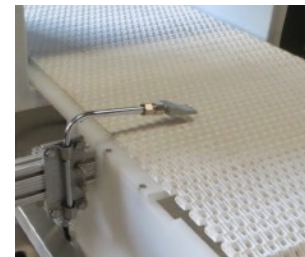
Air Blast Reject
